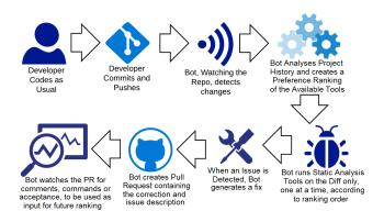
Fig. 1. C-3PR Workflow
